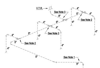
Note 1: The horizontal portion of each individual vent header that exceeds 20'-0" in length shall be increased one pipe size larger than the downstream stack size.
