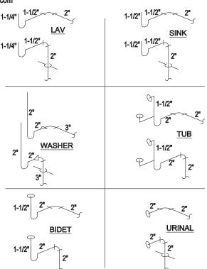
Note: All branch piping located in ceiling or wall areas will be a minium of 2" in size.
