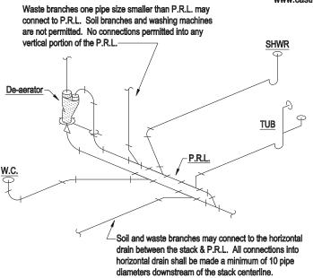
Rough-in height limitations can be reduced by eliminating the Aerator fitting and connecting the lower level fixtures into the horizontal portion of the Sovent system as shown. The De-aerator fitting may be installed above the finish floor providing it remains within 5'-0" of the horizontal drain.
