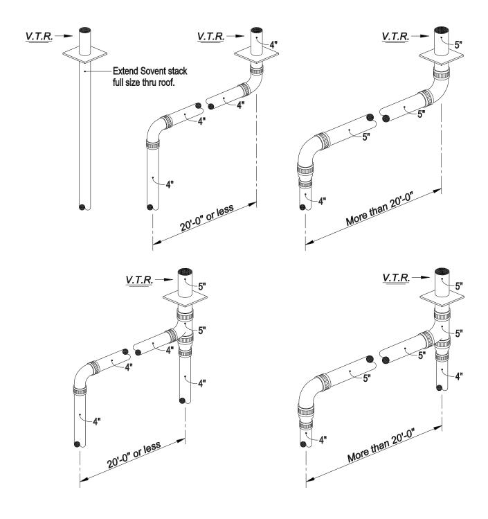
DRAWING NO. 7 Vent Stack Offset Requirements
