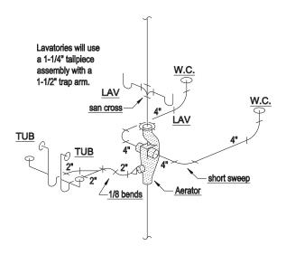
Lavatories will use a 1-1/4" tailpiece 2' assembly with a san tee 1-1/2" trap arm. LAV SHWR combo W.C. 4" Aerator wye TUB (short sweep 1/8 <u>bend</u>
