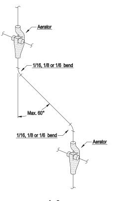
A-8 SOVENT STACK OFFSET - METHOD "A"
