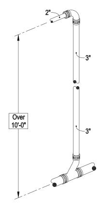
DRAWING NO. 19 Branch Sizing - Vertical Drops
