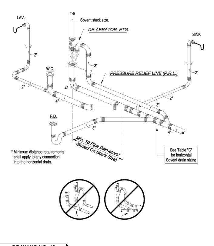
DRAWING NO. 10 Base Of Stack Connections
